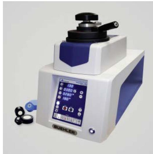
SimpliMet™ 4000 is a new mounting press developed by Buehler – ITW Test & Measurement GmbH ([www.buehler.com](http://www.buehler.com)) for speedy and reliable hot compression mounting of up to two metallographic samples at a time, measuring from 25 mm up to 50 mm in diameter, making it ideal for demanding industrial
